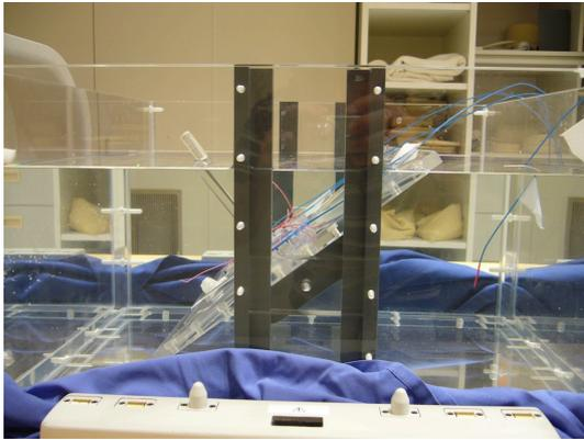
(a) Side view of phantom with object carrier and reference temperature probe in the background.
