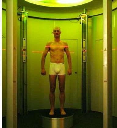
Figure 4.5.: 3D Laser Body Scanner (Vitronic).
