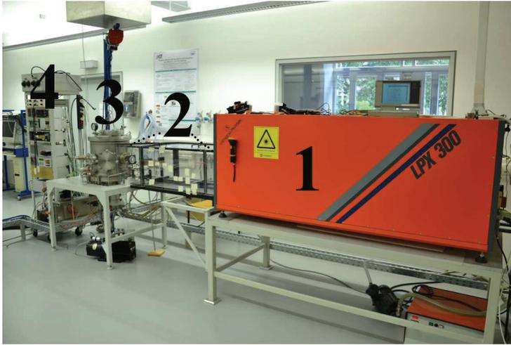
Fig. 4.1.: PLD setup at IMS: The UV light is emitted by the excimer laser (1), guided via mirrors to a lens (2) which focuses the light onto the target in the vacuum chamber (3). The electronics (4) are used to control the deposition process.
