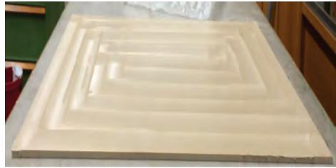
(b) Milled PEEK plate with required thickness
