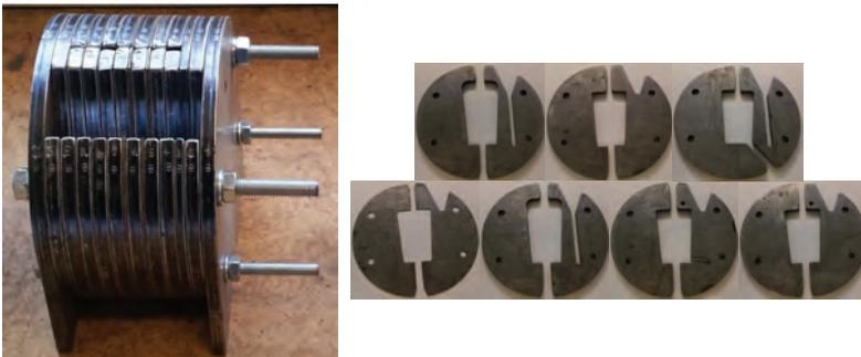
Figure 9.2. Assembled casting form and steel plates
