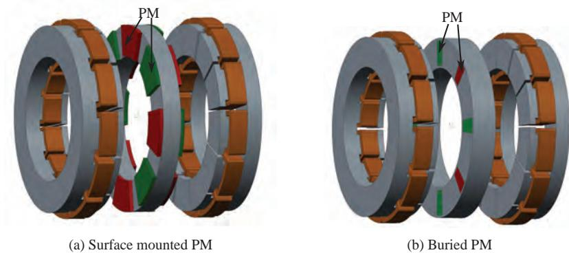
Figure 2.5. PMAFM-IR with surface mounted and buried PMs
