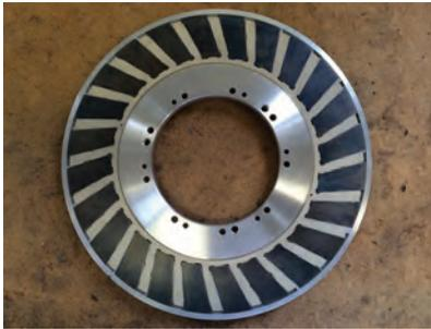
(a) Glued components of rotor
