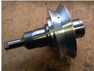
(b) Shrunk shaft and shaft sleeve
