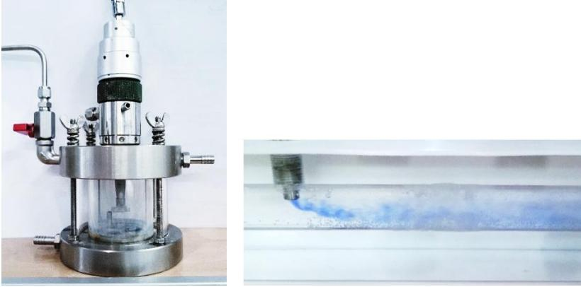
Figure 8.19: Pictures of the experimental reaction compartments  $R_1$ ; left: ST reactor, right: JIC using ink for the flow visualization.
