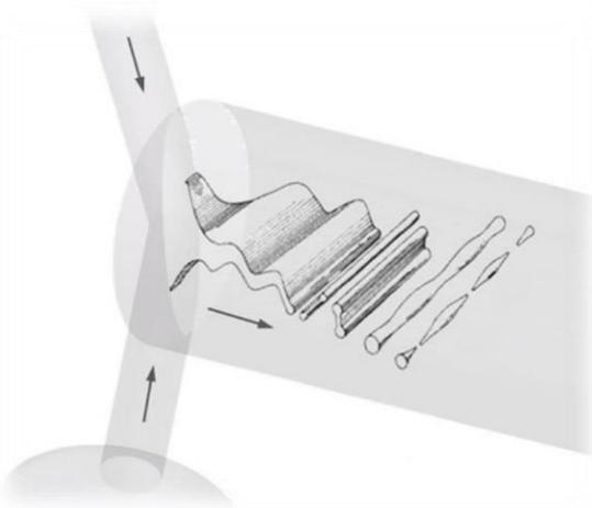
Figure 3.5: Conception of the oscillating mixing structure in the Y-CIJM. (Graphic adaption of the wavy structure from Dombrowski and Johns [60])
