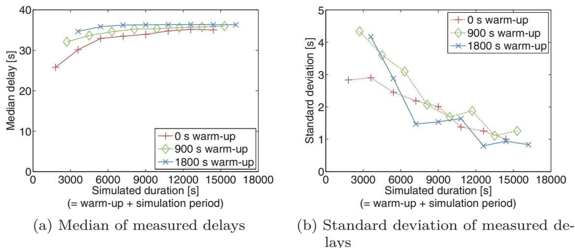
Figure 6.6: Influence of the simulated duration on measured delays for a signal plan in oversaturated conditions (based on 100 replications)
