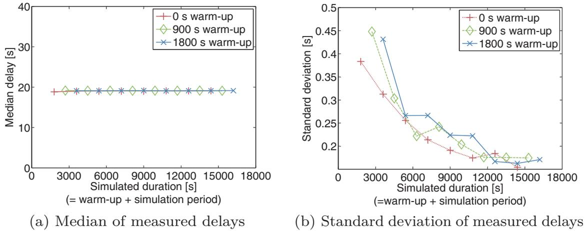
Figure 6.5: Influence of the simulated duration on measured delays for a signal plan in undersaturated conditions (based on 100 replications)
