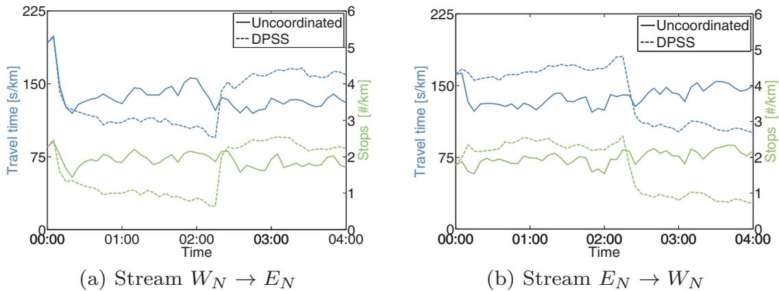
Figure 7.8: Travel time and stops for uncoordinated and coordinated signalisation (DPSS) within selected streams
