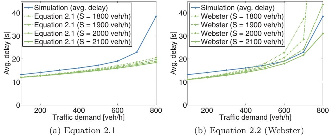
Figure 2.5: Comparison of average delays measured in a microscopic simulator or calculated using approximation formulas ( $t_C = 70$  s,  $t_g = 30$  s)
