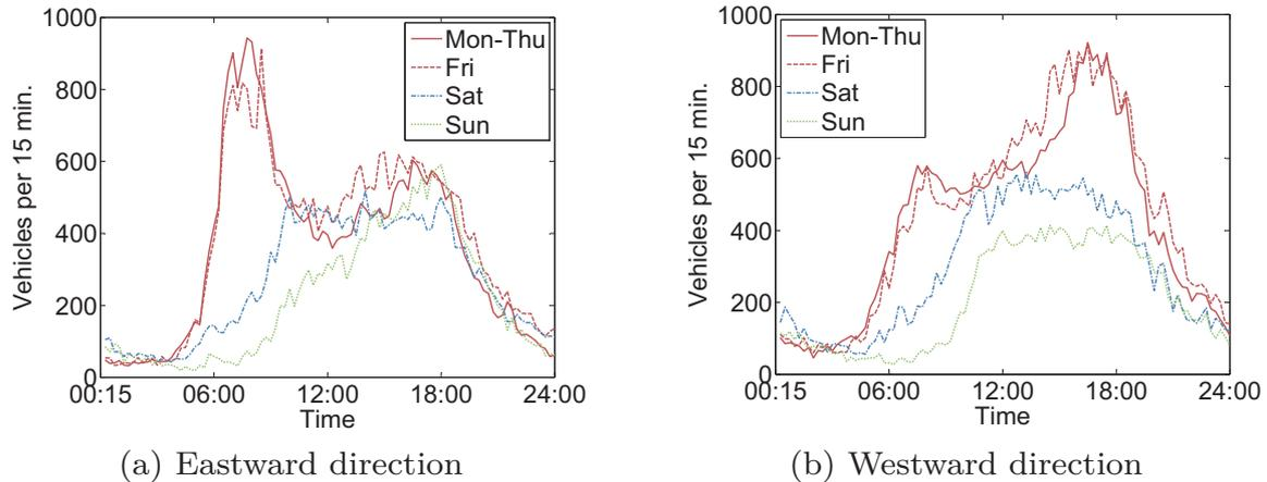
Figure 1.1: Traffic demand of the Südtangente at Karlsruhe, Germany (Data provided by Tiefbauamt Karlsruhe)
