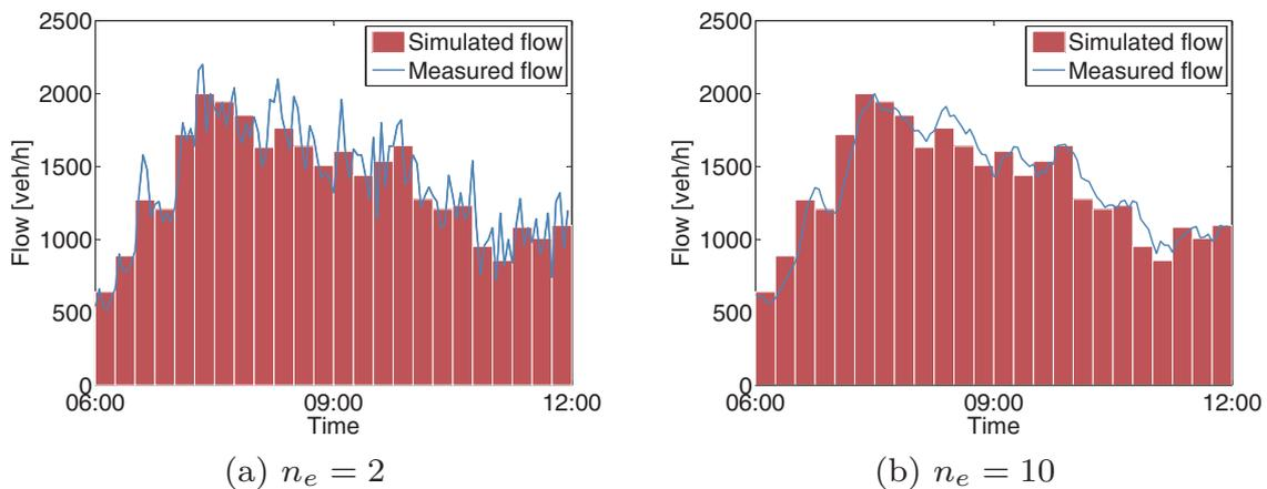
Figure 5.2: Simulated and measured traffic flows for a signal group
