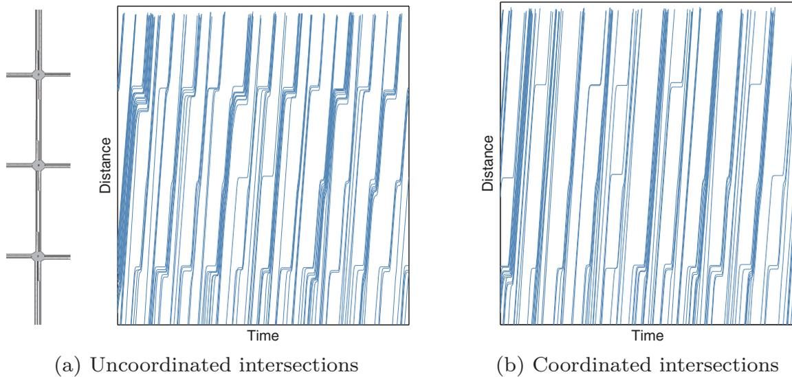
Figure 1.4: Time-distance diagram for an arterial road
