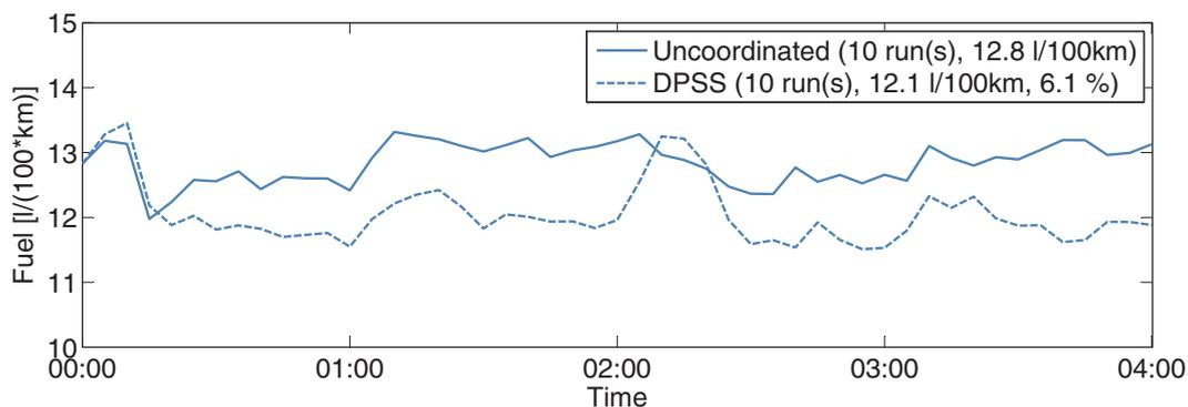
Figure 7.9: Fuel consumption for uncoordinated and coordinated signalisation (DPSS) in a Manhattan network
