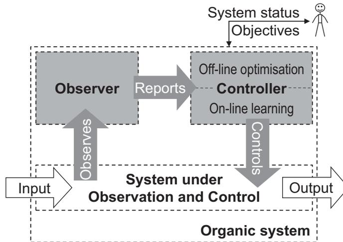
Figure 1.5: Simplified observer/controller architecture
