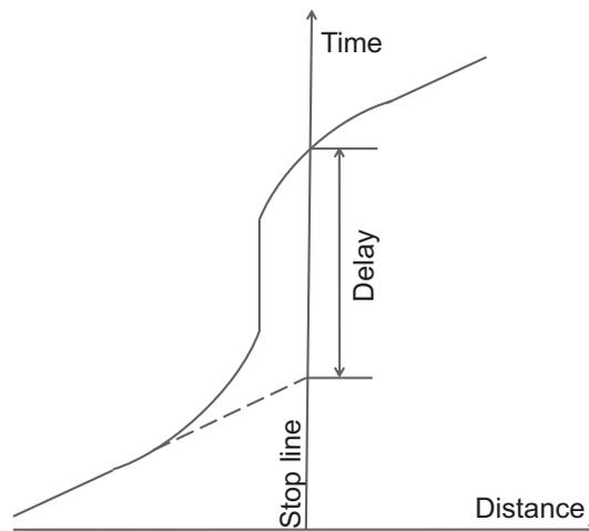
Figure 2.4: Delay of a vehicle at a signalised intersection (based on [171])
