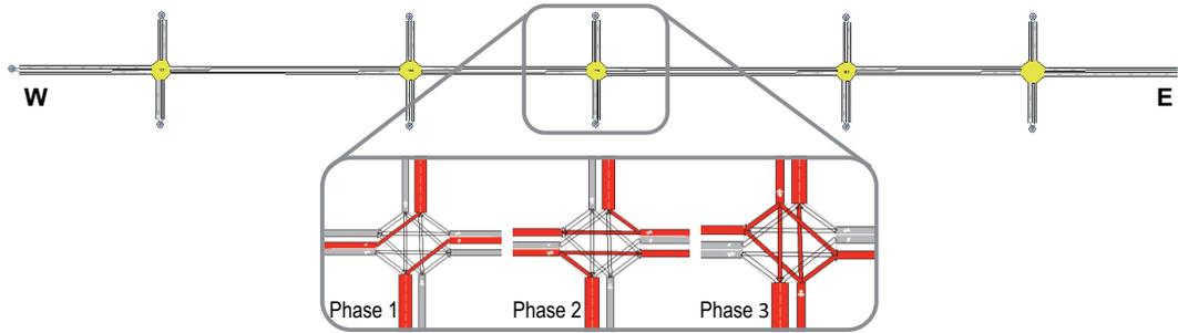
Figure 7.3: An arterial road with three-phased intersections
