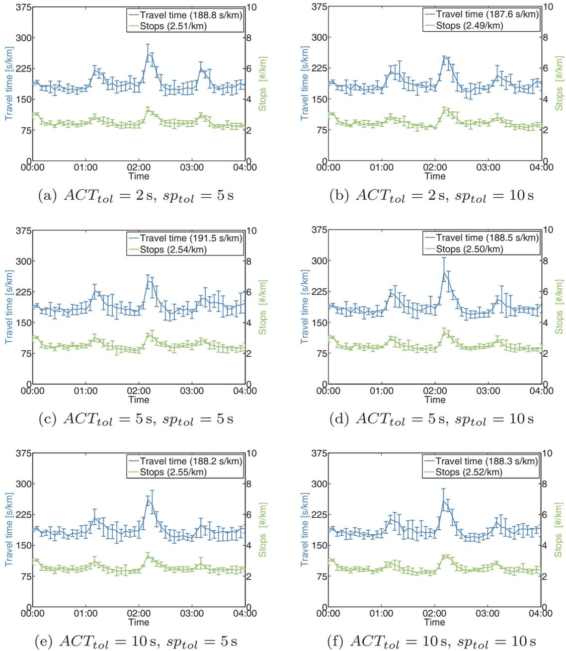
Figure 7.5: Travel times and stops for the arterial road network
