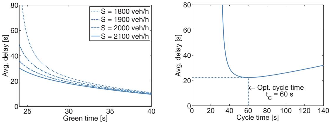
(a) Average delay for a turning depending on the green time ( $t_C = 70$  s,  $M = 600$  veh/h) (b) Average delay for an intersection depending on the cycle time (Two-phased intersection,  $M_1 = M_2 = 600$  veh/h,  $S_1 = S_2 = 1800$  veh/h,  $t_{g,1} = t_{g,2} = 0.5 \cdot t_C - 5$  s)
