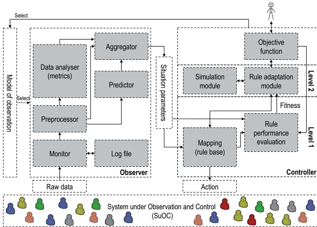
Figure 4.1: Generic observer/controller architecture (based on [159])
