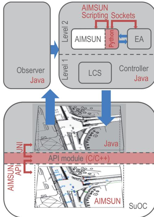
Figure 5.4: Interface between AIMSUN and observer/controller
