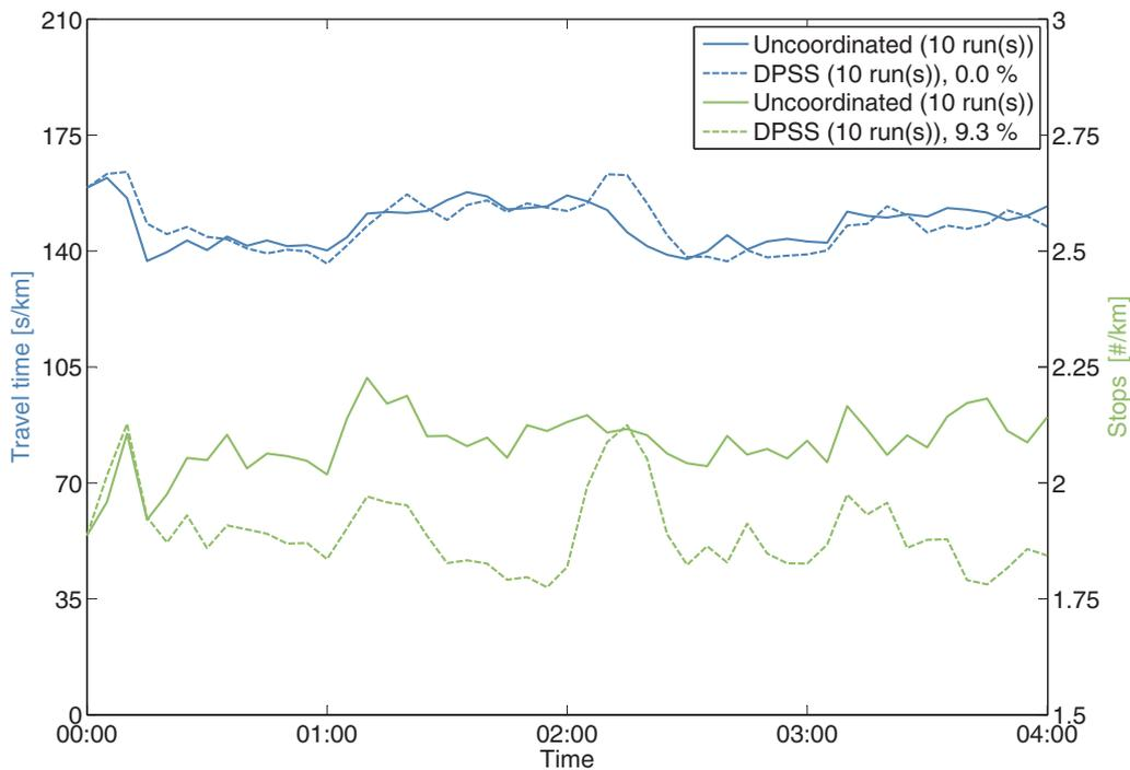
Figure 7.7: Travel time and stops for uncoordinated and coordinated signalisation (DPSS) in a Manhattan network
