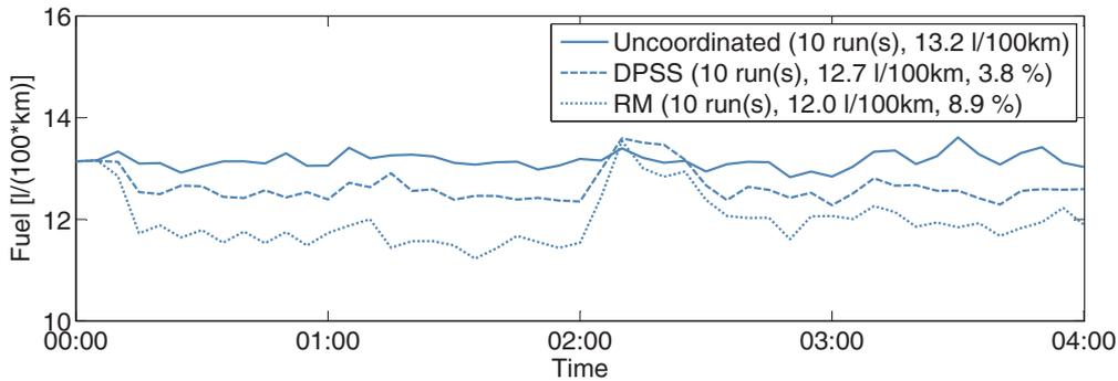
Figure 8.8: Fuel consumption for uncoordinated and coordinated signalisation (DPSS/RM) in a Manhattan network
