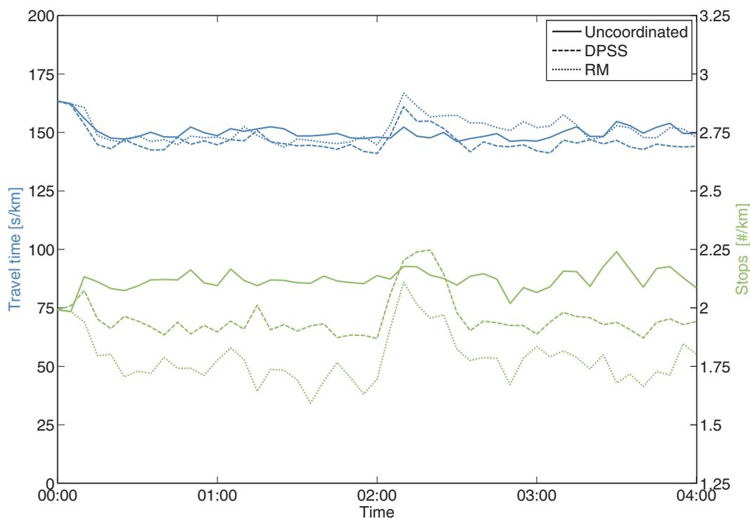
Figure 8.5: Travel time and stops for uncoordinated and coordinated signalisation (DPSS/RM) in a Manhattan network
