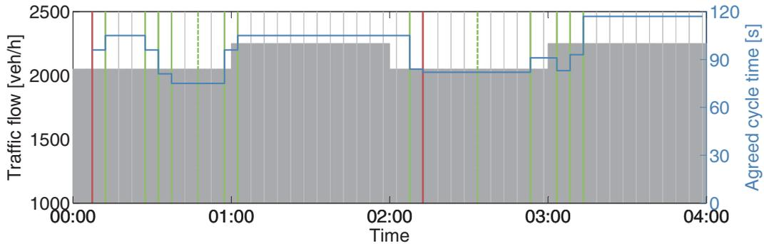
Figure 7.4: Coordination updates for the arterial road network (5 min check frequency,  $ACT_{tol} = 5$  s, and  $sp_{tol} = 10$  s)
