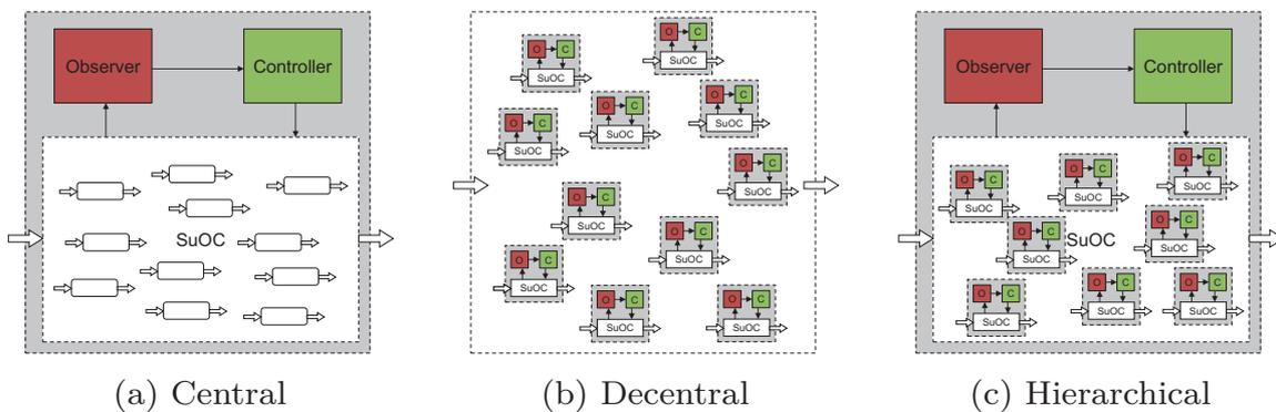
Figure 7.1: Distribution schemes for the observer/controller architecture (based on [23])
