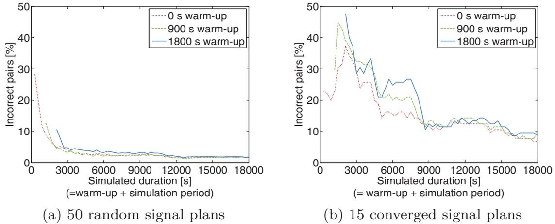
Figure 6.7: Influence of the simulated duration on the ranking of signal plans
