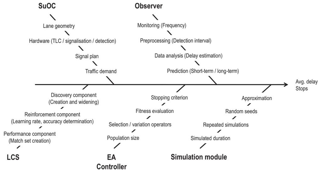
Figure 6.3: Simplified cause-effect diagram for the observer/controller
