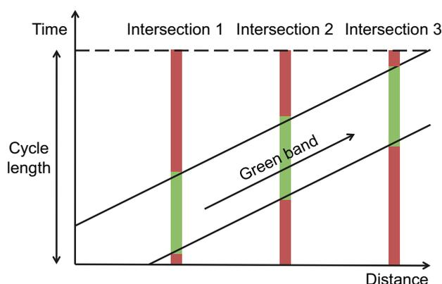
Figure 2.3: Coordination of traffic signals
