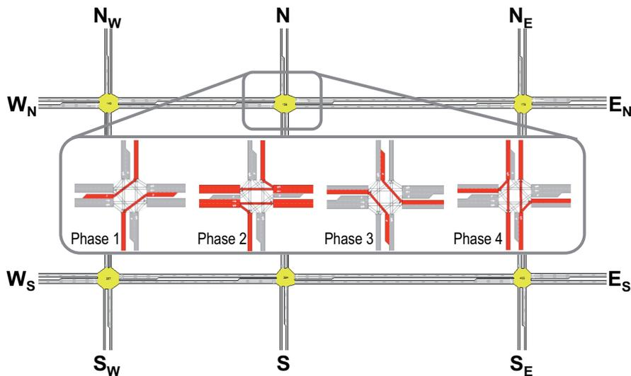
Figure 7.6: A Manhattan network with four-phased intersections
