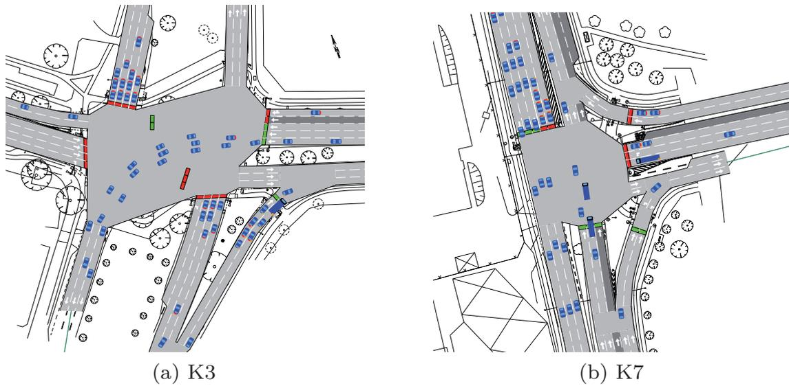
Figure 6.1: Simulation models of Intersections K3 and K7
