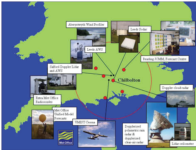
Figure 4.1: Map showing locations of instruments deployed in southern Britain during CSIP. Positions of the radiosonde stations (red circles), from left to right; Bath(B), Swanage(S), Larkhill(L), Chilbolton(C), Reading(R), and Preston Farm(P) (Adapted from Browning et al. 2007).
