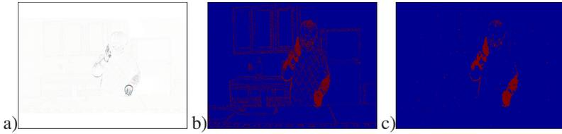
Figure 4.3.: Example for frame based differences showing a) the simple (inverted) difference between two frames with darker values indicating larger differences, b) the simple threshold mask and c) the mask image after morphological post processing
