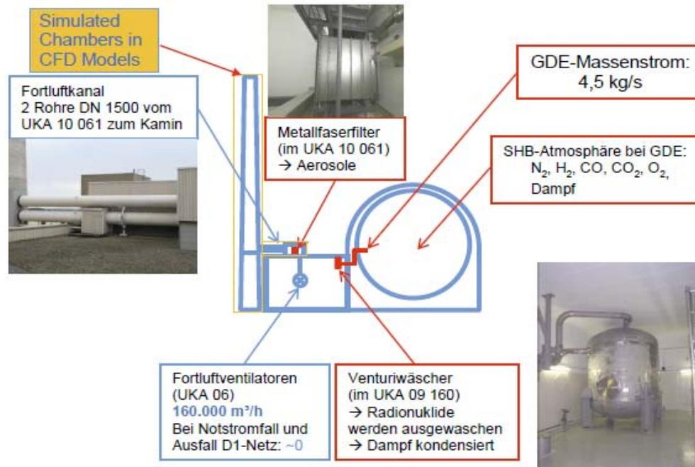
Fig.4: Containment filtered venting system as analysed with GASFLOW
