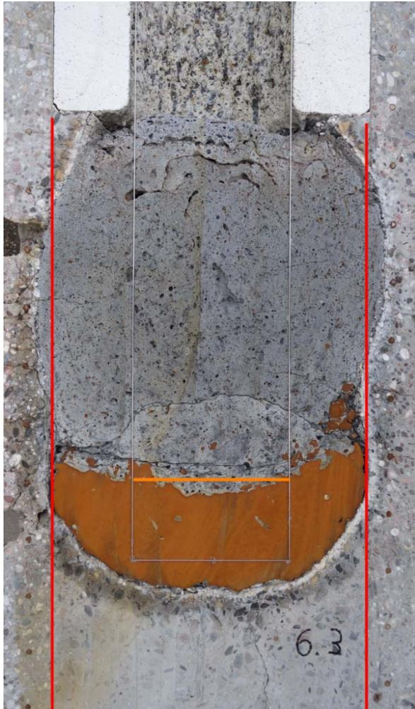
Fig. 4: Section of the MOCKA 6.3 concrete crucible with an indication of the initial size of the crucible. The orange line indicates the initial height (13 cm) of the metal melt and the red line marks the outer surface of the LCS cylindrical crucible.
