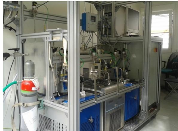
Fig. 11: Measurement of scale and released gases at the geothermal power plant Unterhaching [7].
