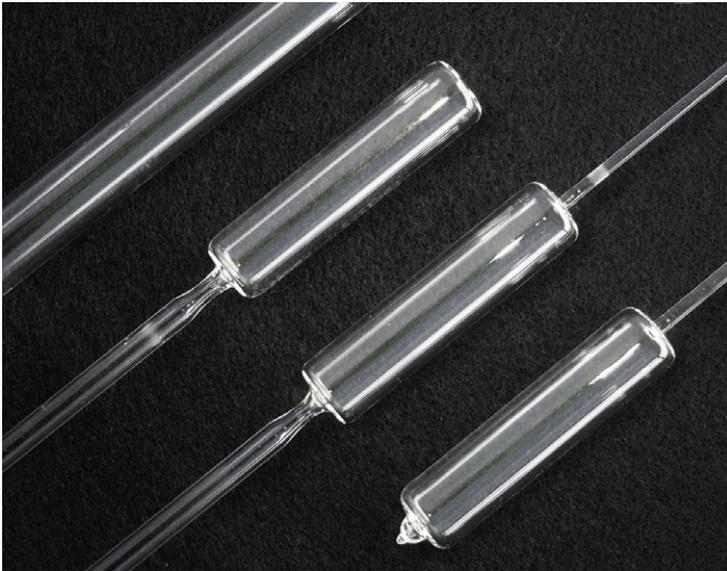
**Figure 6.7:** Individual steps of the lamp production. Fused silica tubes are fused planar on one side, while the other side is narrowed and extended with a filling stem. A glass rod is fused axially to the planar surface to simplify the accurate positioning of the lamp inside the surfatron. After the filling, the lamps are sealed by fusing the filling stem.
