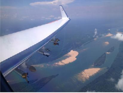
**Figure 6.1.:** The SID-3 instrument (instrument with white cover installed on the centre pylon) onboard HALO over the Amazonian rainforest.
