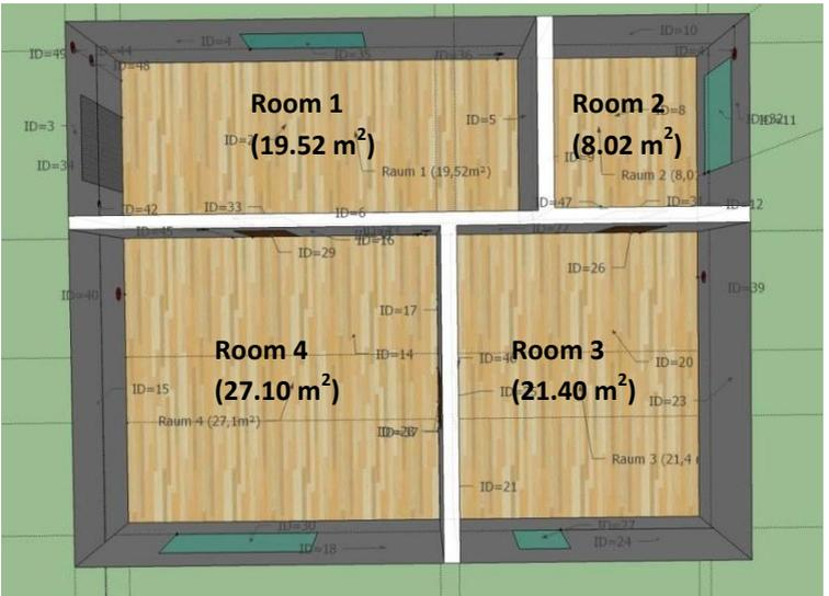
Figure 5-2: Vertical projection (floor plan) with the room numbers and their floor area [m<sup>2</sup>] in the Google SketchUp model for the exemplary four-room apartment (case study 1)
