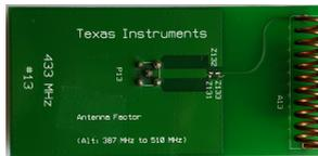
**Figure 3.12:** Photo of the off-the-shelf helix antenna.
