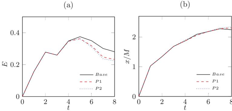
Figure A.11: Kinetic energy at the center of the forced region (a), average interface position (b).
