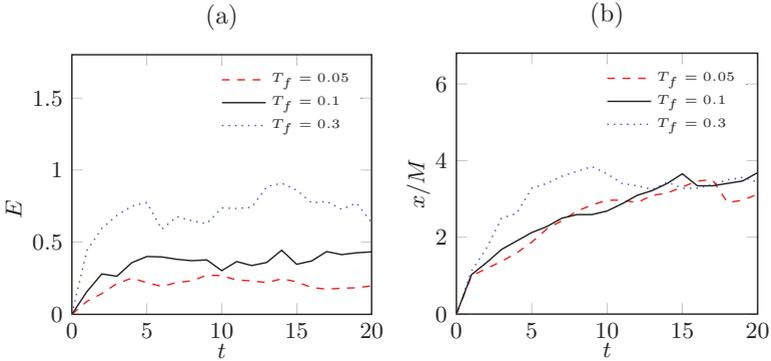
Figure A.2: Kinetic energy in the forced region(a)and average interface position (b).
