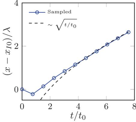
Figure 2.3: Average interface position with respect to time.  $x_{I0}$  denotes the position of the interface at the beginning of the decay. Adapted from [14].
