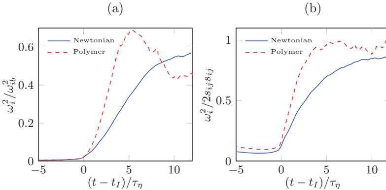
Figure 5.23: Conditional averages in time of entrainment events with respect to the distance from the interface crossing. (a) Enstrophy normalized by the enstrophy in the bulk, (b) ratio between enstrophy and strain.
