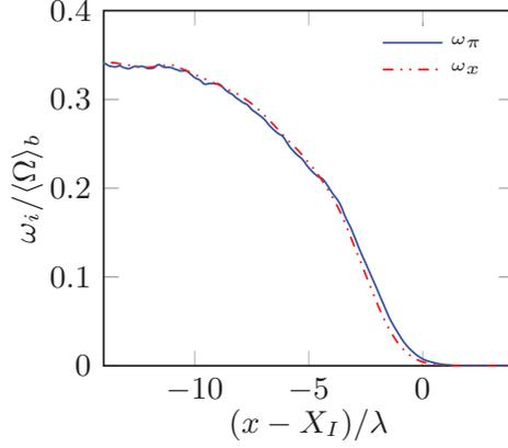
Figure 2.4: Average magnitude of the vorticity components  $\omega_p$  in the homogeneous plane and  $\omega_x$  normal to it as a function of the distance from the average interface position. The value are normalized by  $\langle \Omega \rangle_b$  the average magnitude of the total vorticity in the bulk. Adapted from [14].
