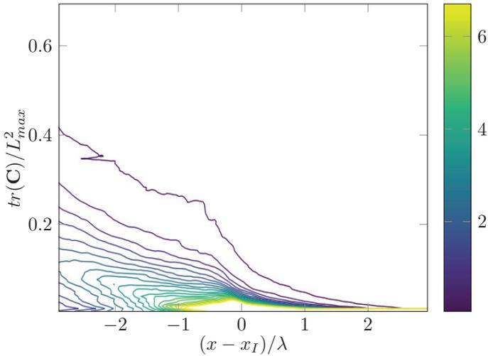
Figure 5.12: Conditional joint probability density function of  $tr(\mathbf{C})/L_{max}^2$  for  $\omega_{i,th}^2 = 0.02\omega_{i,b}^2$
