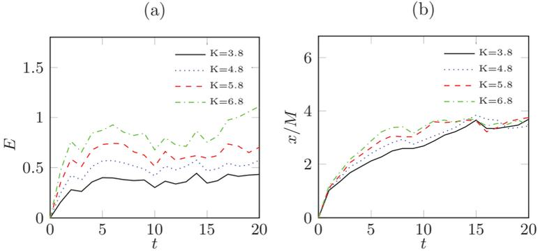
Figure A.1: Kinetic energy in the forced region(a)and average interface position (b).
