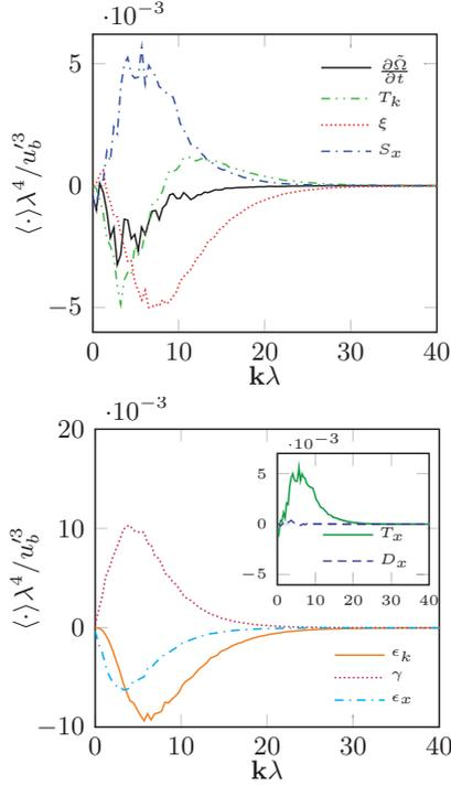
Figure 2.9: Spectral entrophy budget within the inhomogeneous layer at  $(x - X_I)/\lambda = -2$  where the peak of entrophy source due to the spatial flux takes place. The terms of Equation (2.8) are shown in (a) while the different components of  $\xi$  and  $S_x$  from Equation (2.7) are delineated in (b). Adapted from [14].
