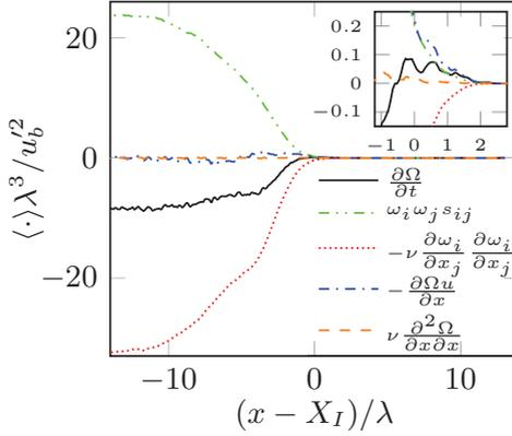
Figure 2.5: Components of the entrophy equations as a function of the distance from the average interface position. The inset is a magnification of the same plot at the interface region. Adapted from [14].
