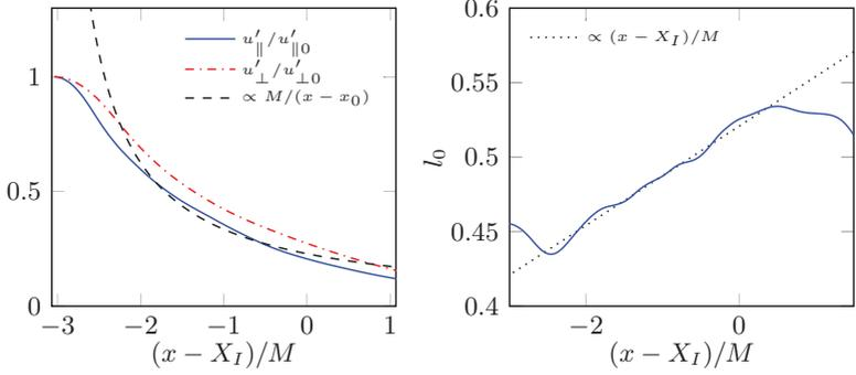
Figure 4.5: (a) Profiles of the magnitude of velocity fluctuations in the direction parallel to the homogeneous planes  $y - z$  and normal to them as a function of the distance from the average interface position. The black dashed line represent the fit with a function inversely proportional to the distance from a virtual origin in the forced region. (b) Variation of the integral length scale as a function of the distance from the average interface position.
