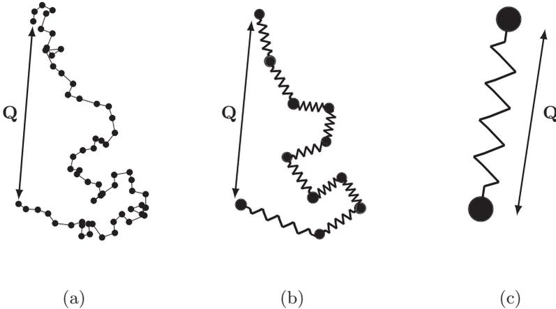
Figure 3.2: Various degrees of simplification of the polymer model with its end-to-end vector  $Q$ . (a) Multi chain dumbbell model with rigid connectors between the beads. (b) Multi-chain dumbbell model with elastic connectors. (c) Single elastic dumbbell model.
