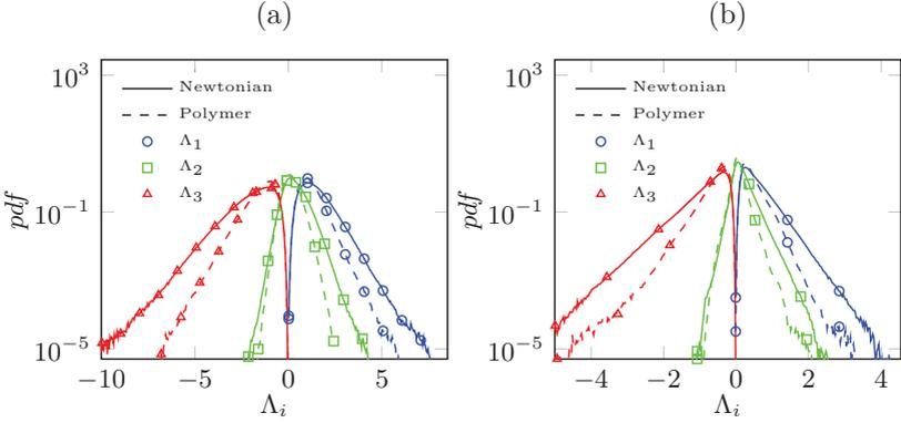
Figure 5.13: Probability density function of the strain eigenvalues  $\Lambda_i$  (a) in the bulk and (b) at the interface. Adapted from [16].
