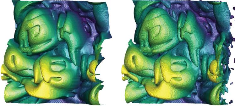
Figure A.13: Example of the interface by two different detection algorithms. Right: only the outermost thresholded points are selected. Left: simplified algorithm from Borrell and Jimenez algorithm prior the removal of pockets and bubbles.
