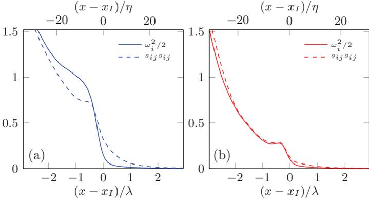
Figure 5.9: Conditional averages of enstrophy compared to the strain rate. (a) Newtonian case, (b) polymers for  $\omega_{i,th}^2 = 0.02$ .
