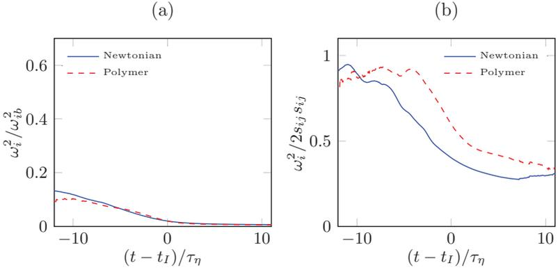
Figure 5.26: Conditional averages in time of extrainment events with respect to the distance from the interface crossing. (a) Enstrophy normalized by the enstrophy in the bulk, (b) ratio between enstrophy and strain.
