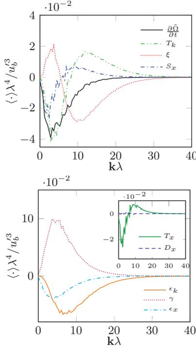
Figure 2.7: Spectral enstrophy budget within the bulk turbulent region for  $t/t_0 = 4.3$ . The terms of Equation (2.8) are shown in (a) while the different components of  $\xi$  and  $S_x$  from Equation (2.7) are delineated in (b). Adapted from [14].
