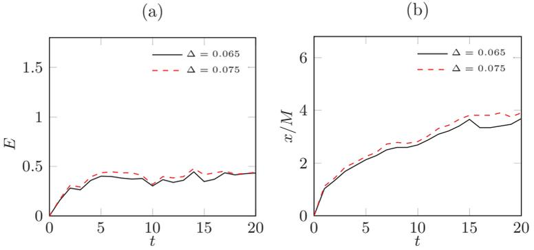
Figure A.3: Kinetic energy at the center of the forced region (a), average interface position (b).
