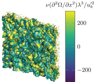
Figure 2.11: Viscous diffusion of enstrophy in a 2D cross-section of the turbulent/non-turbulent interface. Adapted from [14].
