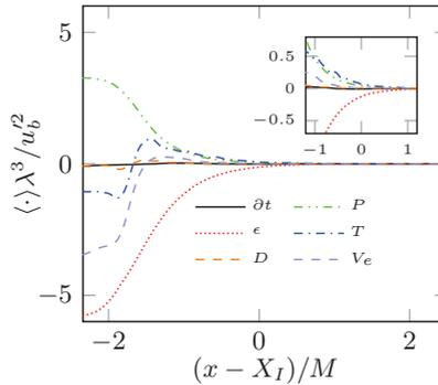
Figure 5.6: Enstrophy budget for the polymer case. The right scale refers to  $f_m$ , i.e. the maximum possible amplitude of the body force.
