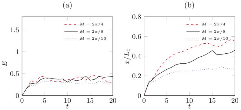
Figure A.4: Kinetic energy at the center of the forced region (a), average interface position (b). In this case for the sake of comparison the interface position has been normalized by the box half size  $L_x$ .
