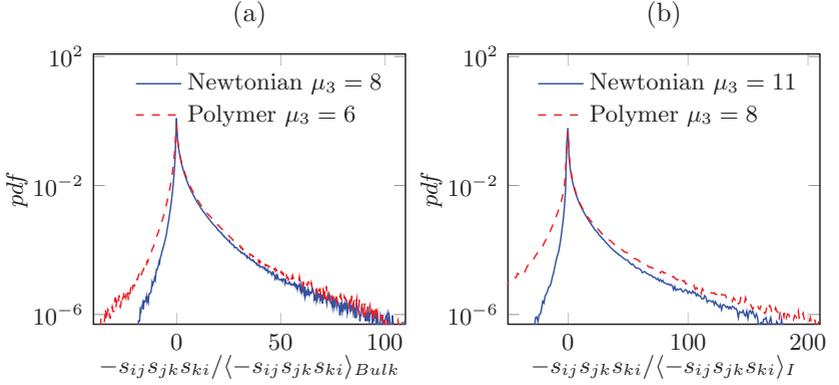
Figure 5.20: Probability density function of the normalized strain rate production  $s_{ij}s_{jk}s_{ki}$  normalized by its average value. (a) in the bulk (b) at the interface,  $\mu_3$  is the estimated skewness of the distribution. Adapted from [16].
