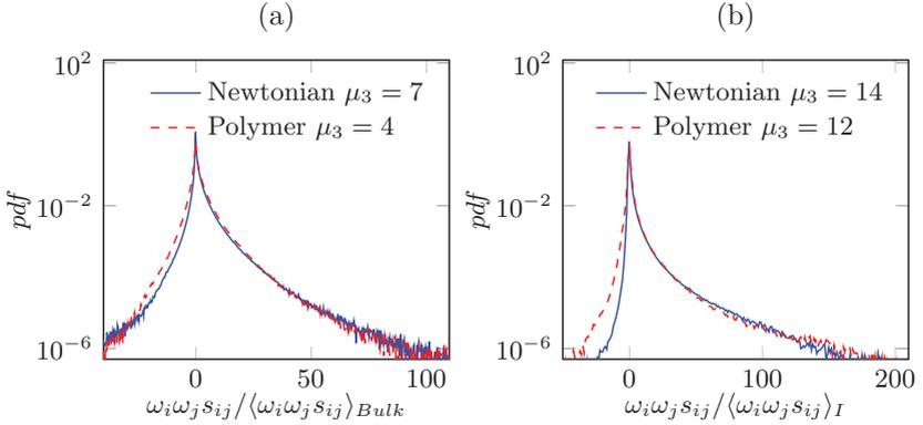
Figure 5.18: Probability density function of the enstrophy production  $\omega_i \omega_j s_{ij}$  normalized by its average value. (a) in the bulk (b) at the interface,  $\mu_3$  is the estimated skewness of the distribution. Adapted from [16].
