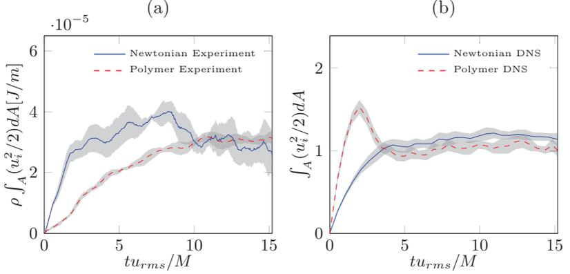
Figure 4.7: Time variation of the integral of the kinetic energy contained in the region between the bulk and the interface. Gray areas mark  $\pm 1.96$  standard errors of the mean. Adapted from [16].
