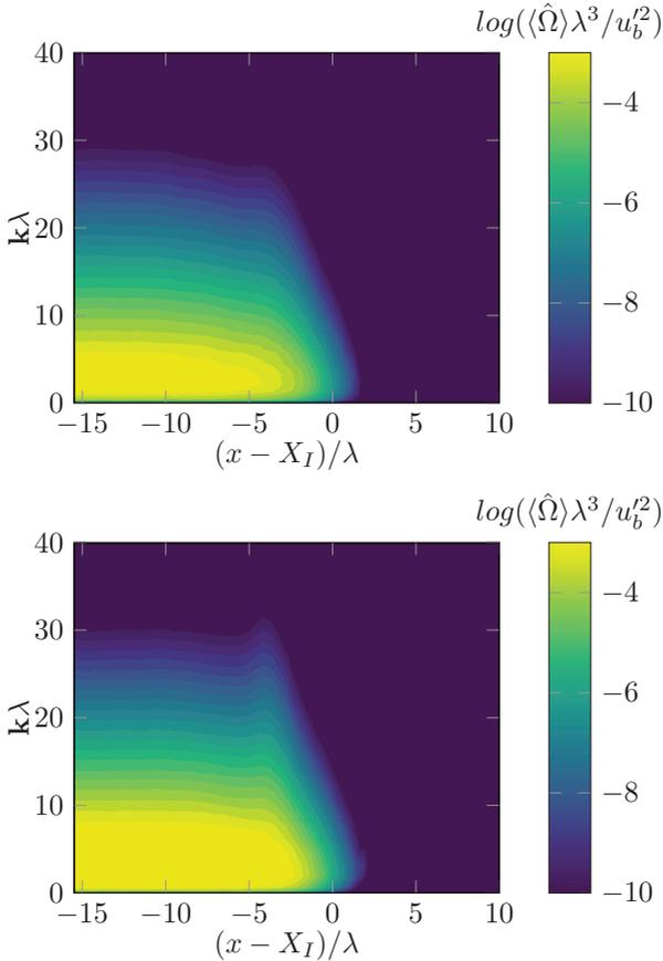
Figure 2.6: Isocontours of  $\log(\langle \hat{\Omega} \rangle \lambda^3 / u_b^2)$  in the  $(k, x - X_I)$ -space for (a)  $t/t_0 = 4.5$  and (b)  $t/t_0 = 8$ . Adapted from [14].
