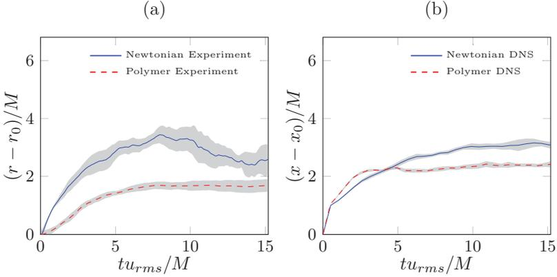
Figure 4.8: Time variation of the average interface position for Newtonian fluid and the dilute polymer solution, comparison between simulation and experimental measurements. The left y-axis refers to the experiments while the right one to the simulations. Grey areas mark  $\pm 1.96$  standard errors of the mean. Adapted from [16].
