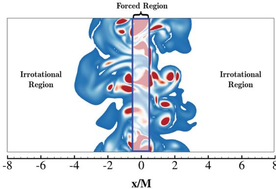
Figure 4.2: Depiction of the computational box with a slice of the enstrophy iso-contour for a Newtonian simulation. Adapted from [16].
