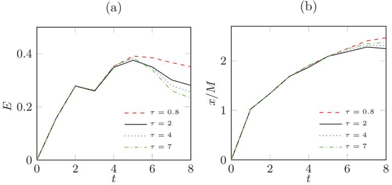
Figure A.6: Kinetic energy at the center of the forced region (a), average interface position (b).
