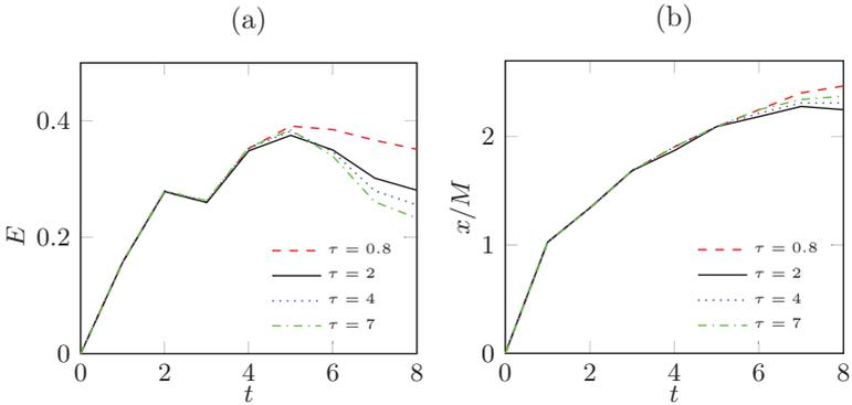
Figure A.10: Kinetic energy at the center of the forced region (a), average interface position (b).
