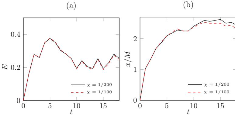
Figure A.8: Kinetic energy at the center of the forced region (a), average interface position (b).
