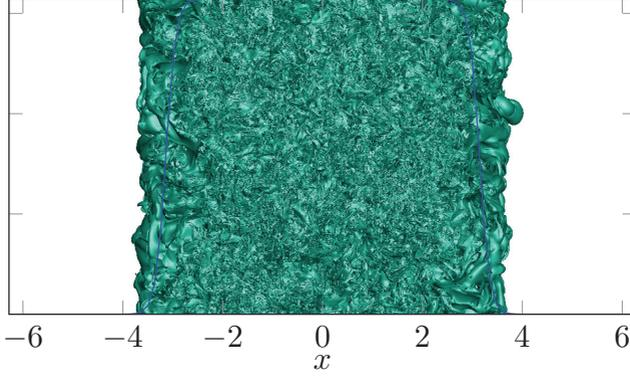
Figure 2.2: The smoothing function from Equation 2.4 superimposed over plotted iso-surfaces of the enstrophy field.
