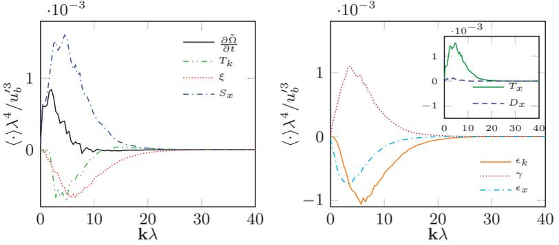
Figure 2.10: Spectral enstrophy budget within the interfacial layer at  $(x - X_I)/\lambda = 0$  for  $t/t_0 = 4.3$ . The terms of Equation (2.8) are shown in (a) while the different components of  $\xi$  and  $S_x$  from Equation (2.7) are delineated in (b). Adapted from [14].
