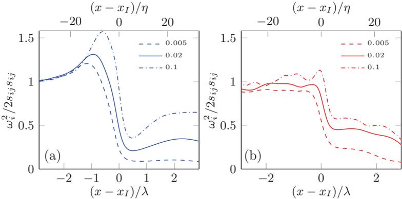
Figure 5.10: Conditional averages of the ratio  $\omega_i^2/2s_{ij}s_{ij}$  for three different thresholds  $\omega_{i,th}^2 = 0.1 - 0.02 - 0.005\omega_{i,b}^2$ . (a) Newtonian case, (b) polymers.
