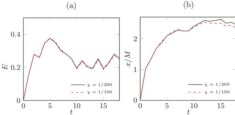
Figure A.12: Kinetic energy at the center of the forced region (a), average interface position (b).
