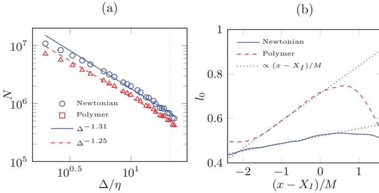
Figure 4.11: (a) Number of boxes  $N$  containing portion of the interface against box size  $\Delta/\eta$ . The dotted line marks the box of size  $\Delta = M$ . (b) Integral length scale as a function of the distance from the interface.
