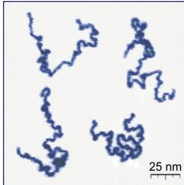
Figure 3.1: An atomic force microscope picture of a poly(2-vinylpyridine) ( $n \times C_7H_7N$ ) chain of about 1500 monomers at different degrees of un-coiling [72].
