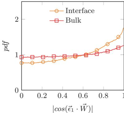
Figure 5.17: Probability density function of the cosine of the angle between the largest conformation tensor eigenvector  $\vec{e}_1$  and the vortex stretching vector  $\vec{W} = \{\omega_j s_{ij}\}$ .
