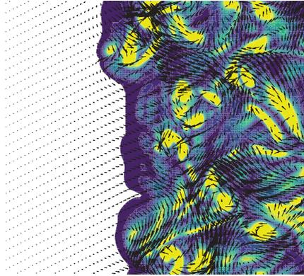
Figure 2.1: Velocity field vectors (arrows) superimposed over isocontour of  $\omega_i^2/2$  in a DNS of a propagating turbulent front. The color cut-off level is set at 2% of the average enstrophy in the turbulent bulk of the flow.
