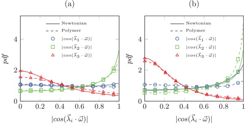
Figure 5.14: Probability density function of the cosine of the angle between the vorticity vector and the three strain eigenvector  $\vec{\lambda}_i$ . (a) in the bulk, (b) at the interface. Adapted from [16].
