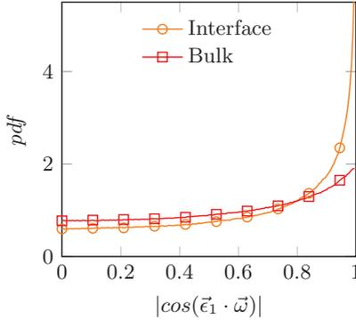
Figure 5.16: Probability density function of the cosine of the angle between the largest conformation tensor eigenvector  $\vec{e}_1$  and the vorticity vector. Adapted from [16].
