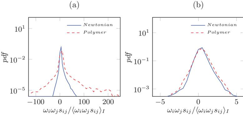
Figure 5.28: Probability density function of the normalized enstrophy production from the Lagrangian tracers at the interface crossing. (a) Entrainment events, (b) extrainment.
