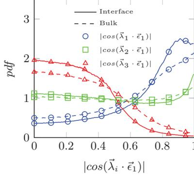
Figure 5.15: Probability density function of the cosine of the angle between the largest conformation tensor eigenvector  $\vec{e}_1$  and the three strain eigenvector  $\vec{\lambda}_i$ . (a) in the bulk, (b) at the interface. Adapted from [16].
