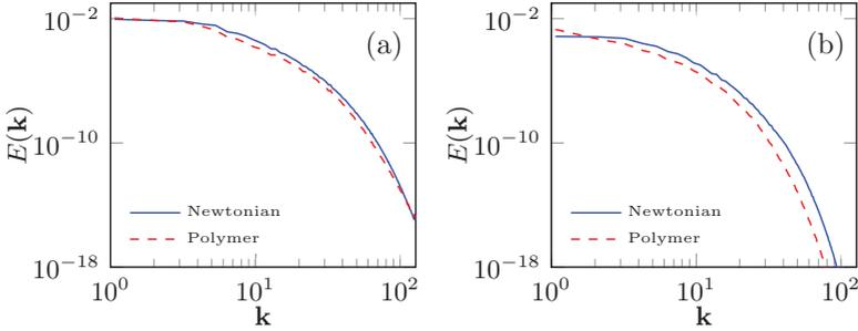
Figure 5.1: Spectra of kinetic energy compute over homogeneous planes  $y - z$  in the bulk (a) and at the average interface position (b).
