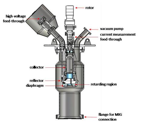
**Fig. 1.8.1:** Representation of the prototype diagnostic device that was manufactured for the study of the beam quality of magnetron injection guns.
