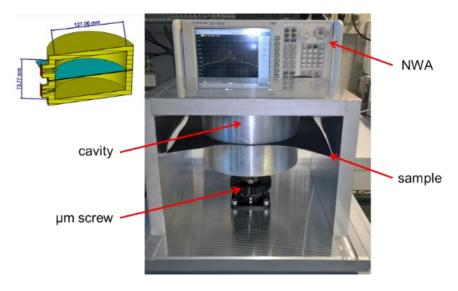
Fig. 4.2.1: Dielectric measurements setup for thin multilayer materials at 2.45 GHz.
