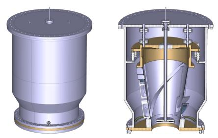
Fig. 1.3.7: Drawings of the preliminary conceptual design of a two-stage E×B MDC.
