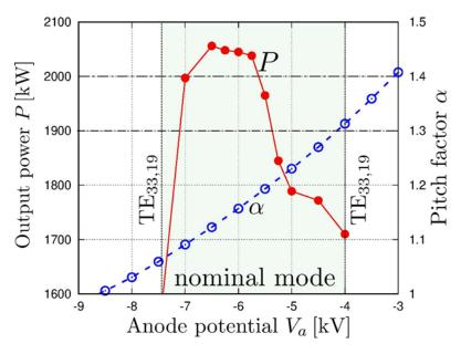
Fig. 1.4.2: Experimental measured output power P and theoretical pitch factor α as functions of the modulation anode potential.
