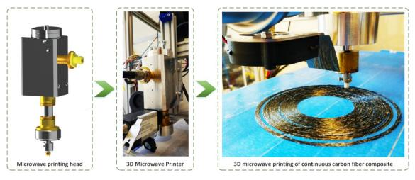
Fig. 4.7.1: 3D microwave printing technology of continuous carbon fiber reinforced composites.
