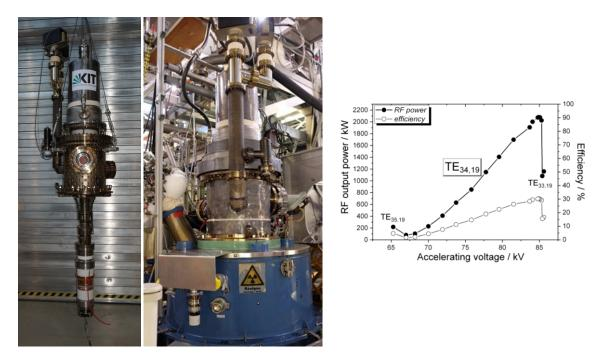
**Fig. 1.3.1:** left: longer-pulse coaxial gyrotron assembly with old diode gun before (left) and after (middle) installation in the superconducting magnet. Right: measured power and efficiency versus the applied accelerating voltage.
