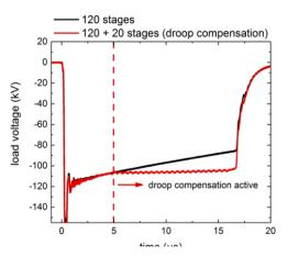
**Fig. 2.2.3:** Output voltage of the generator with droop compensation (red) in comparison to a pulse shape without droop compensation (black).
