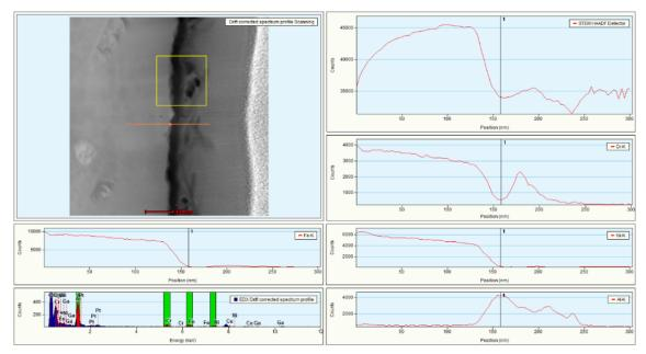
Fig. 2.3.2: TEM, EDX investigation of alumina forming HEA after 2000 exposure to Pb at 600°C
