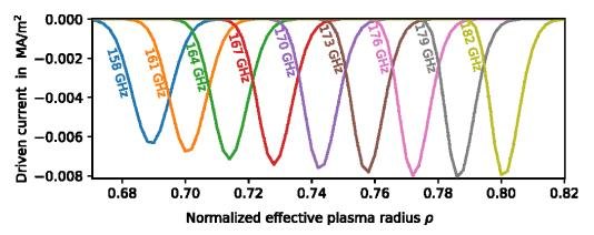
**Fig. 1.3.8:** Illustration of a first simulation of the localized current drive from the equatorial port of EU DEMO achieved at different frequencies.
