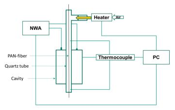
Fig. 4.4.1: Schematic of the set up for conventional heating and measurement of the dielectric properties.
