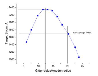
Fig. 3.1.1: Target current of GESA IV as function of the ratio of grid to anode radius.
