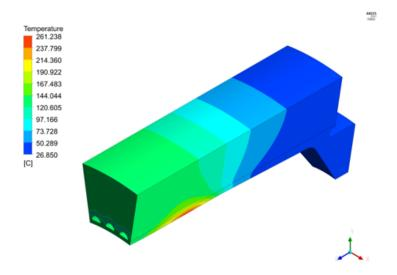
Fig. 1.3.2: Temperature profile on the cavity wall (18 degrees section) and heat sink with the proposed mini-channels.
