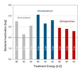
Fig. 2.1.1: Inactivation of bacteria isolated from electrocoating lines by PEF-treatment with 1  $\mu$ s and 2  $\mu$ s long pulses at a specific treatment energy of 40 kJ/l and 80 kJ/l.
