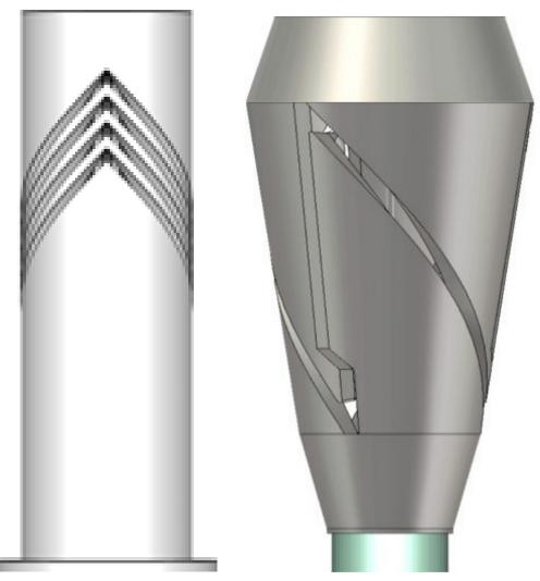
Fig. 1.3.6: A coaxial four stages MDC at (left) and a cylindrical two stages MDC (right).
