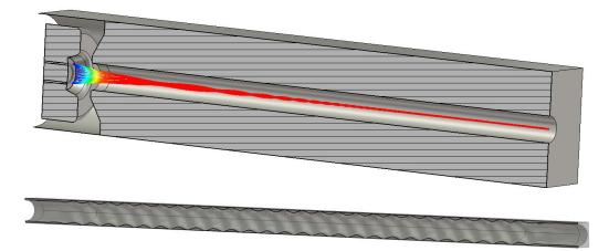
**Fig. 1.7.1:** CUSP-type electron gun with beam tunnel, to be attached to a helical gyro-TWT (top). Cross-section of a helical waveguide structure for a helical gyro-TWT (bottom).
