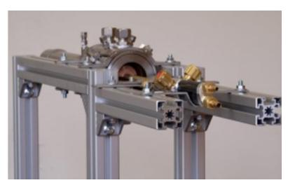
Fig. 1.3.3: Test set-up for the performance analysis of the mini-channel cooling concept.
