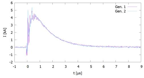
Fig. 2.2.1 shows the well synchronized pulse currents of both generators after triggering.
