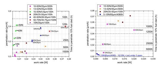
**Fig. 3.1.2:** Penetration rate vs working rate for different fretting conditions in molten PbBi with  $10^{-7}$ wt% oxygen at 400°C; left side without long-term test / right side: with long-term test.
