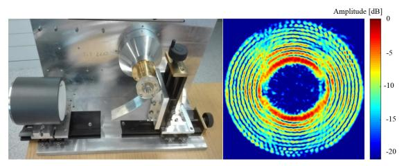
Fig. 1.1.1: Mode generator for the  $TE_{28,10}$  mode (top) and measured normalized pattern (electric field amplitude – vertical polarization) of  $TE_{28,10}$  at 140.155 GHz (bottom).
