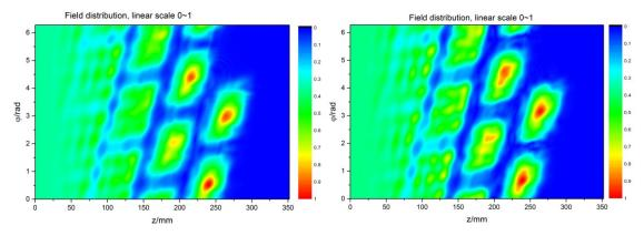
**Fig. 1.3.5:** Field distribution on the launcher wall (linear scale  $0^{-1}$ ): operating in the TE<sub>34,19</sub> mode at 170 GHz (left) and in the TE<sub>40,23</sub> mode at 204 GHz (right).
