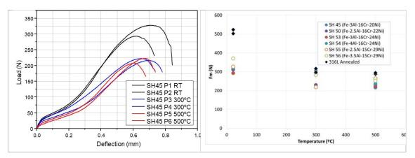
Fig. 3.1.3: Small punch test of AFA alloys showing the ductile behaviour of the new developed material.
