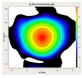
Fig. 1.1.2: The field distribution on the gyrotron window.
