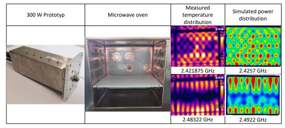
Fig. 4.3.1: Prototype of a 300 W solid state microwave source, Microwave oven and comparison of measured and simulated modes
