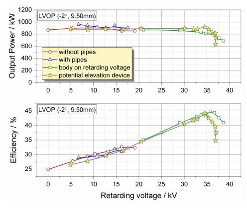
Fig. 1.2.2: RF power and total efficiency vs. retarding voltage obtained experimentally with different gyrotron configurations.
